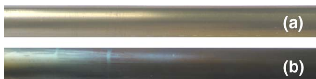
Fig. 6. Photographs of the Zircaloy surfaces after the deposition experiments at 200 °C in (a) suspended hematite solution and (b) mixed solution consisting of \text{Fe}^{2+} ions and hematite colloidal particles.
